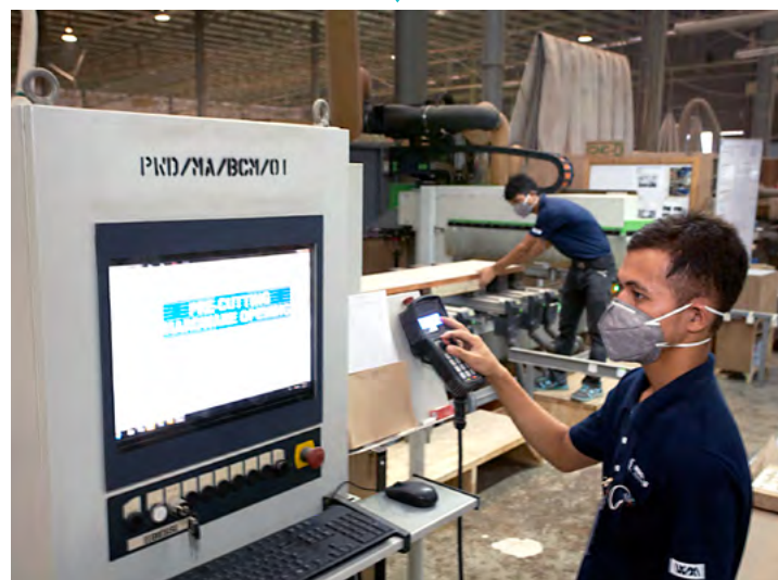
Processing hardware precutting with CNC machine
